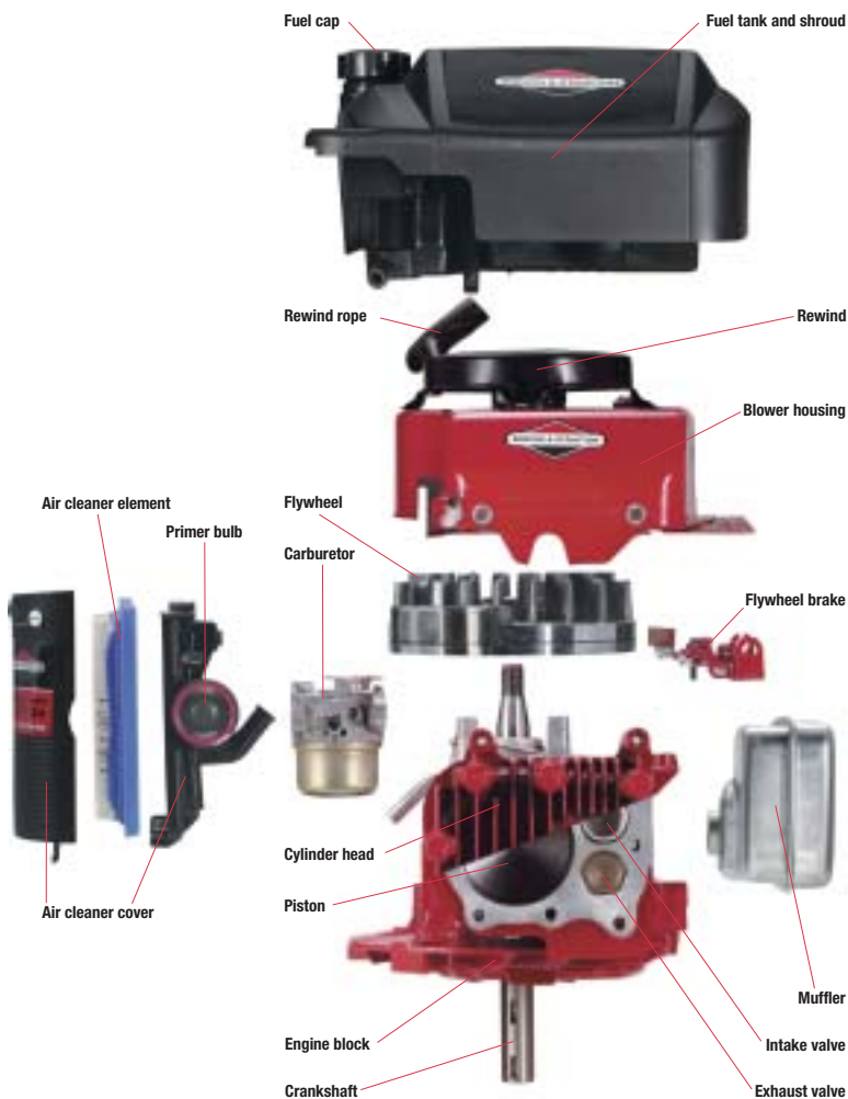
Parts of the small engine – front view
